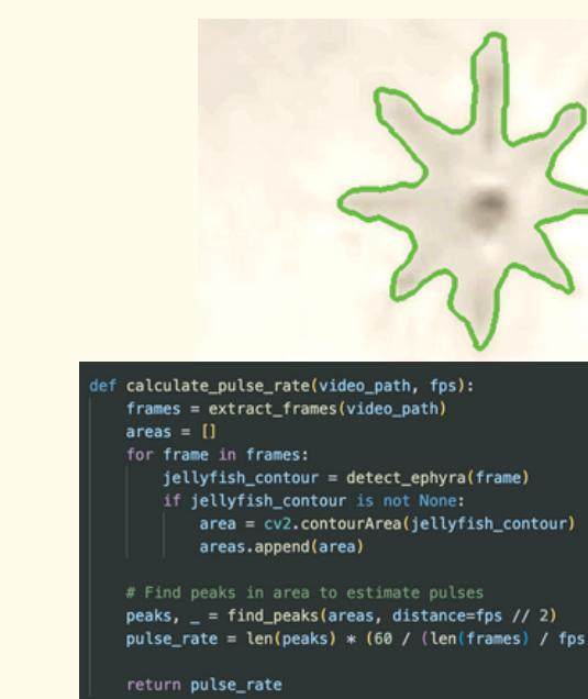
Figure 2. Our code used OpenCV to draw contours around the jellyfish and detected changes in area to count pulses.
