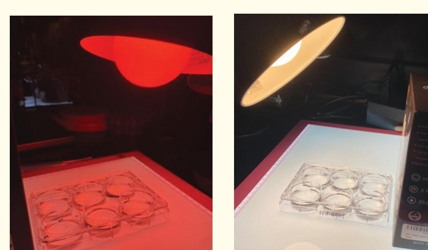
Figure 1. Our experimental setup consisted of 6-well plates, a light board, and lamps with different colored bulbs (white/yellow and red). Plates were stored on a shaker when we were not collecting data/training.
